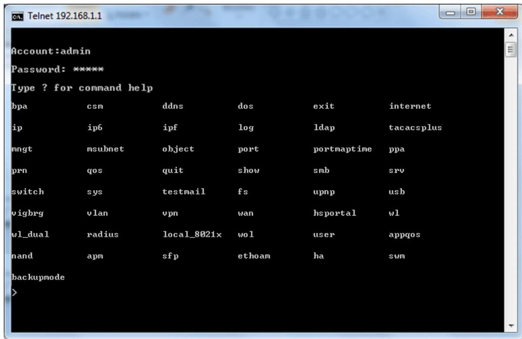
For users using previous Windows system (e.g., 2000/XP), simply click Start >> Run and type Telnet 192.168.1.1 in the Open box as below. Next, type admin/admin for Account/Password. And, type ? to get a list of valid/common commands.
