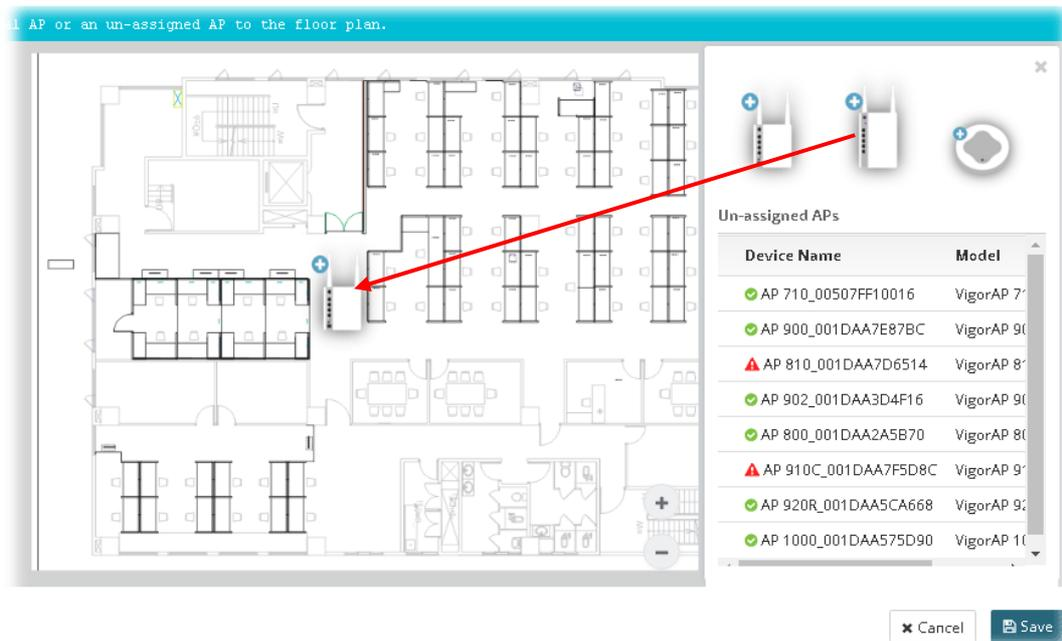
8. Choose one of device names from the list of Un-assigned APs. Drag the device name to the icon on the left side.
