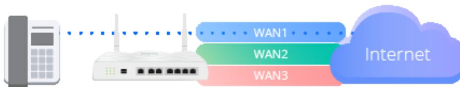
Digital phones can be connected to any router via Ethernet interface (no need to support VoIP function). With the VoIP WAN function, we can set a range. As long as the signal strength falls within this range, you can use digital phones to communicate with the remote end.
