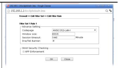
Codepage - This function is used to compare the characters among different languages. Choose correct codepage can help the system obtaining correct ASCII after decoding data from URL and enhance the correctness of URL Content Filter. The default value for this setting is ANSI 1252 Latin I. If you do not choose any codepage, no decoding job of URL will be processed. Please use the drop-down list to choose a codepage.
