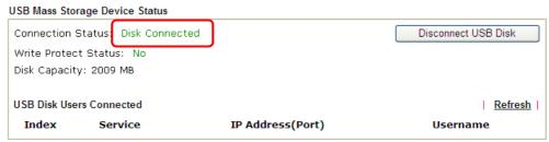
Note: If the write protect switch of USB disk is turned on, the USB disk is in READ-ONLY mode. No data can be written to it.
