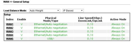
Note: The line speed setting of WAN interface is available only when According to Line Speed is selected as the Load Balance Mode.
