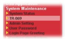
3. In the field of ACS Server, type the URL (IP address with port number) of Vigor3220 Series and type the same Username and Password defined on the page of Central VPN Management>>General Setup in Vigor3220 Series. Then, click Enable for CPE Client and then click OK to save the settings.
